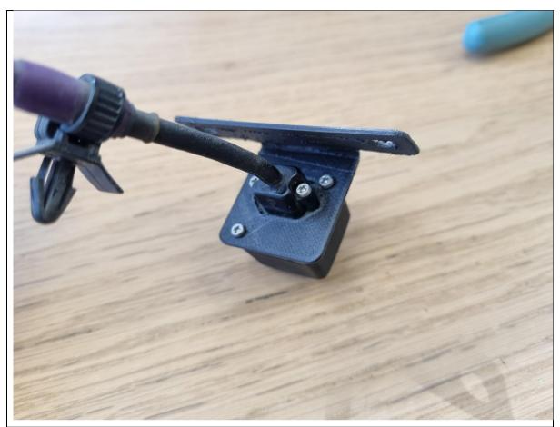
8. Re-connect the camera harness to the camera using the 2x factory Phillips head screws from previous.
